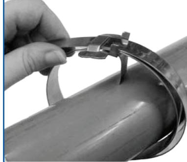
Continue band around object once more and again through buckle. Double banding develops a great deal more radial compression than single banding. Bend end of band under buckle.
