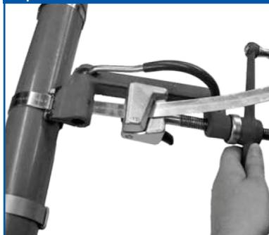
Roll tool over buckle, backing off with tension handle throughout entire rolling operation. Failure to back off with tension handle through-out entire course of roll-over may result in breaking of band. There is no loss of tension as band released is used up in the bend.
