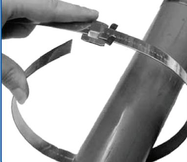
Band may be used from bulk roll as this completely eliminates waste of band. Slide buckle on band as shown, bringing end of band around object to be clamped and again through buckle.
