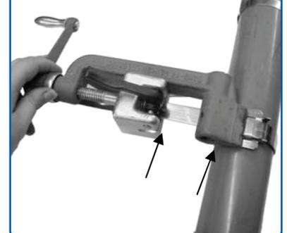
Place band in opening of tool nose and gripper block. Move into slot as far as possible, to avoid buckle sliding into tool nose. Tighten band clamp by turning the tension handle clockwise while holding band gripper tight against band. *NOTE: The spring load of the band gripper is not intended to secure and prevent band from slipping during tension process.*
