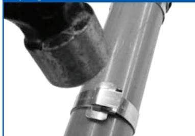
Hammer down buckle ears to hold band stub in place to complete BANDIT clamp
